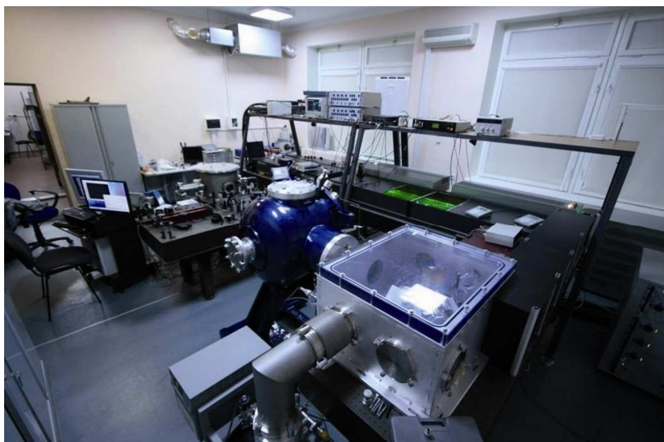
Fig. 4. Femtosecond multiterawatt Ti:sapphire laser system in the JIHT RAS (800 nm, 30 fs, 10 Hz, 10 TW)
