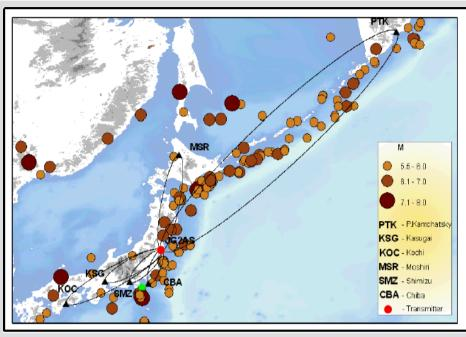
A schematic of radio transmitter and receivers in the Japan-Russia system together with earthquake (M>5.5) epicenters in the period 2000-2003.
