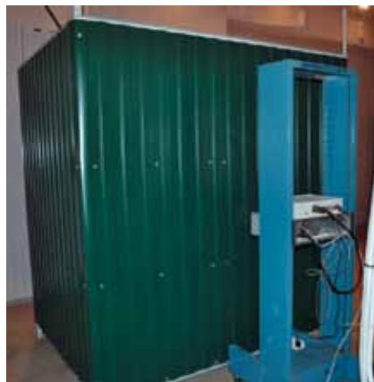
**Detector of hazardous materials scanning through container with hidden illicit material**
