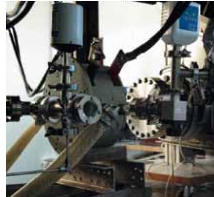
Plasmachemical reactor for deposition of extremely high-enriched 28Si isotope thin film
